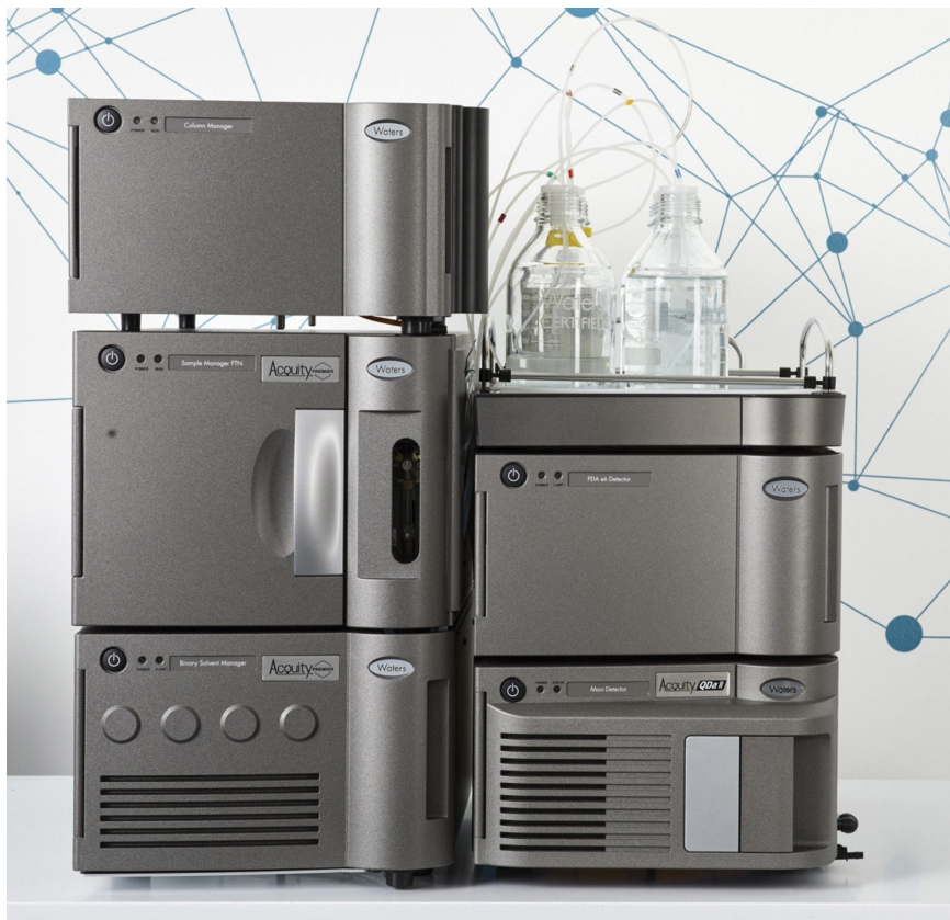
Figure 1. The ACQUITY QDa II Mass Detector and ACQUITY Premier UPLC configuration.
