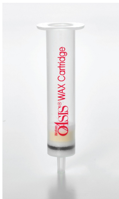
Figure 1. Oasis WAX/GCB for PFAS Analysis Cartridges.
