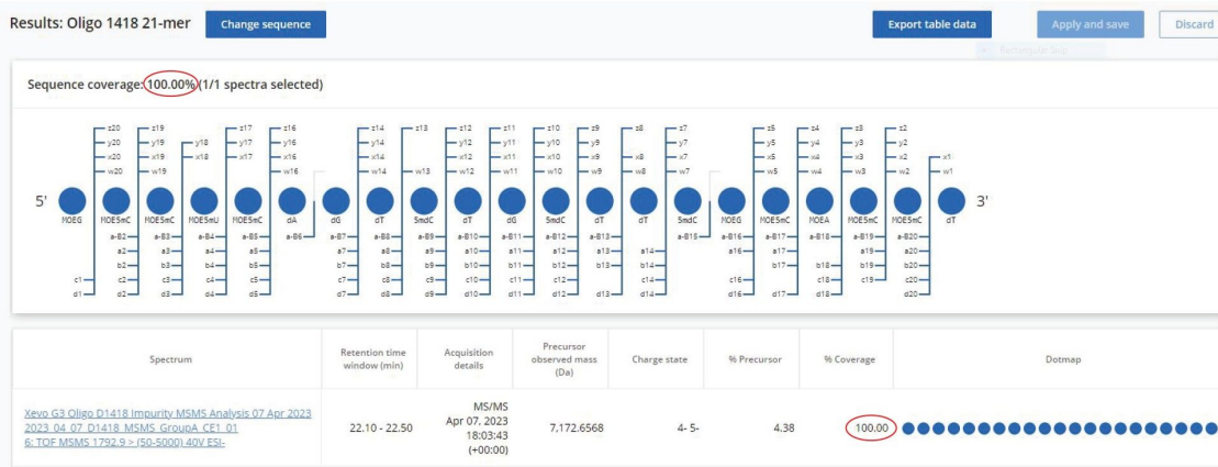
Figure 9. Complete sequence coverage (100%) resulted from the MS/MS fragmentation of the [M-4H]^{-4} precursor ( m/z=1792.14 ) of the 21-mer siRNA oligonucleotide. The precursor was fragmented with an optimized fixed collision energy (40 V) in the collision cell of a Xevo G3 QTof mass spectrometer.
