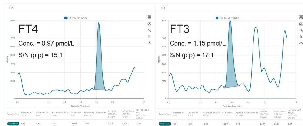
Figure 4. Typical chromatograms of FT4 and FT3 spiked in dialysate, extracted, and analyzed.
