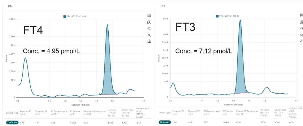
Figure 3. Typical Chromatograms of FT4 and FT3 from human serum samples which have been dialyzed, extracted, and analyzed.
