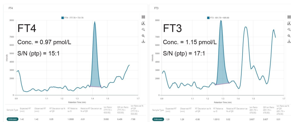
Figure 4. Typical chromatograms of FT4 and FT3 spiked in dialysate, extracted, and analyzed.
