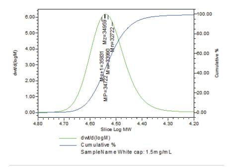
Figure 4. Molecular weight distribution plot for polystyrene sample.
