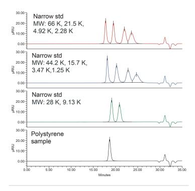
Figure 1. Chromatographic separation of polystyrene standards and sample solutions generated by an Arc HPLC System with a strong solvent compatibility kit and RI detector.
