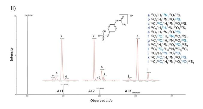
Figure 3. I) 10 Hz UPLC MRT ES- precursor fine isotope spectrum obtained for [acetaminophen sulfate -H]<sup>-</sup> 200,000 FWHM. II) 10 Hz UPLC MRT ES- precursor fine isotope spectrum obtained for [acetaminophen sulfate -H]<sup>-</sup> 300,000 FWHM.
