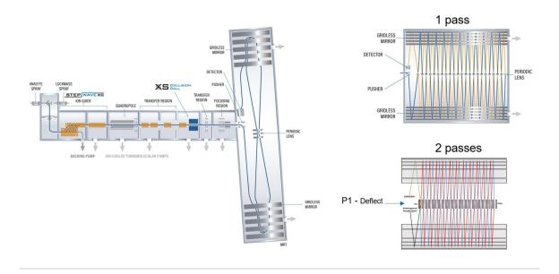
Figure 1. SELECT SERIES MRT instrument schematic illustrating one pass (>200,000 FWHM) and two passes REM mode (>300,000 FWHM).
