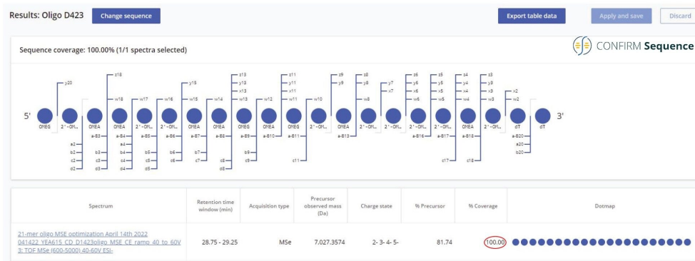
Figure 5. Complete (100%) sequence coverage, presented in a dot-map format, produced by high energy MS E untargeted fragmentation. All precursors of the 21-mer heavily modified oligonucleotide were fragmented using an optimized collision energy ramp (from 40 to 60 V) applied to the collision cell of a Xevo G2-XS instrument.
