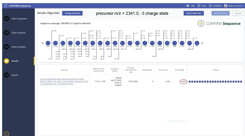
Figure 3. CONFIRM Sequence screenshot showing excellent MS/MS fragmentation coverage (100%) in a dot-map format. The [M-3H]^{-3} precursor of the 21-mer heavily modified oligonucleotide ( m/z = 2342.0 ) was fragmented using an optimized fixed collision energy (set at 63 V) in the collision cell of a Xevo G2-XS QToF instrument.
