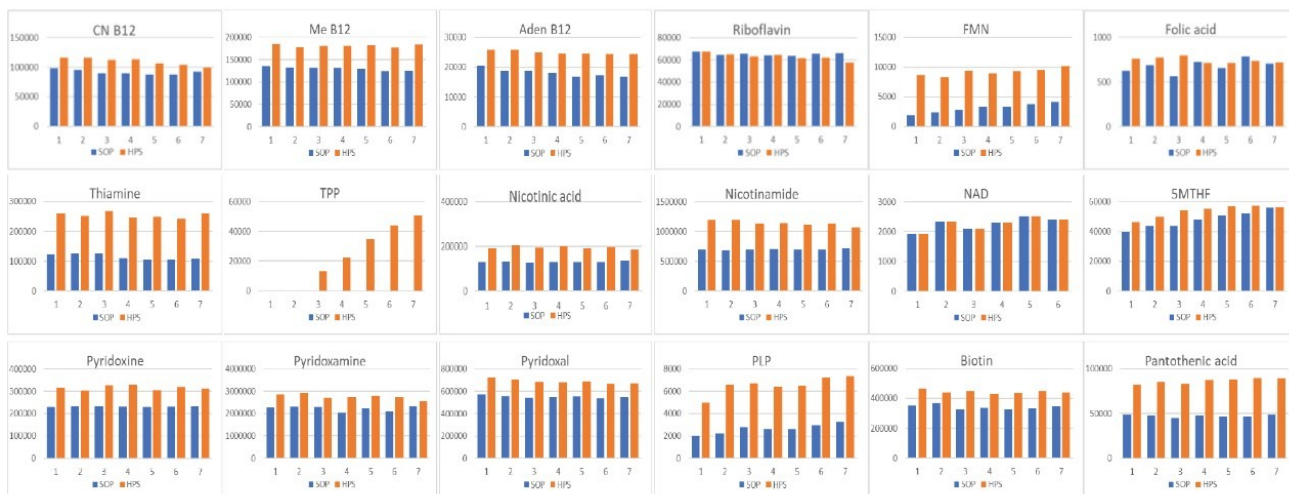
Figure 2. Comparison of LC-MS/MS peak areas of B vitamins and their vitamers with the HPS setup and the SOP setup. Peak areas from stainless steel surfaces (SOP, blue bar) are plotted side by side with those from MaxPeak HPS (HPS, orange bar).
