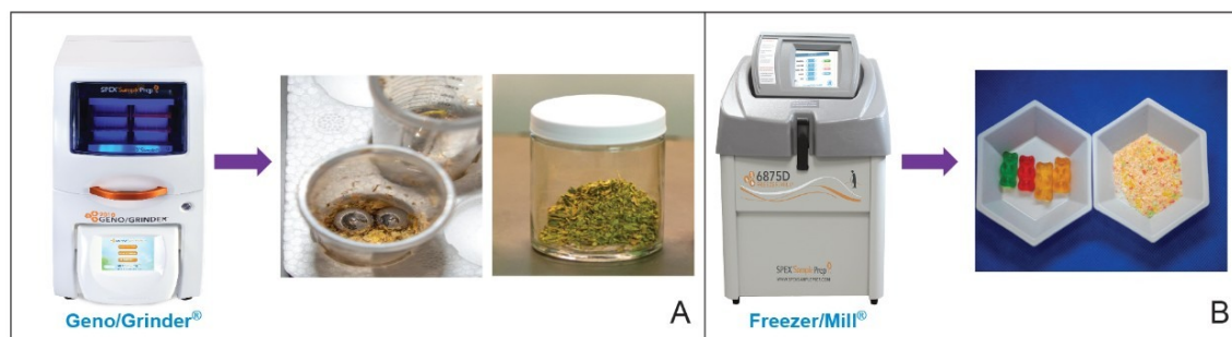
Figure 1. Geno/Grinder® used for solvent extractions of solid material (panel A). The stainless balls facilitate comminution and can be used for shaking during the QuEChERS extraction. The Freezer/Mill® is used to pulverize gummy and sticky materials (panel B).
