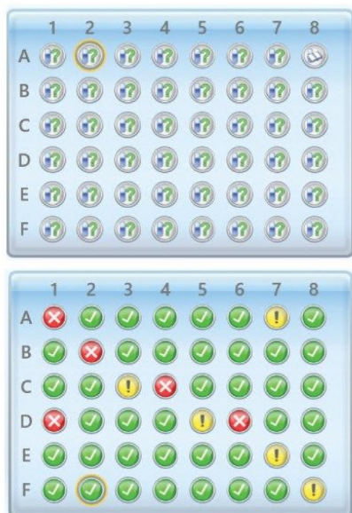
Figure 6. Mass confirmation status for each sample on a 48 vials plate before and after the automated data acquisition and processing in waters_connect.
